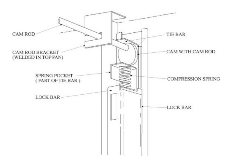
If cabinet is locked, a 3/8" or ½" drill bit should be used to drill into the center of the lock.
